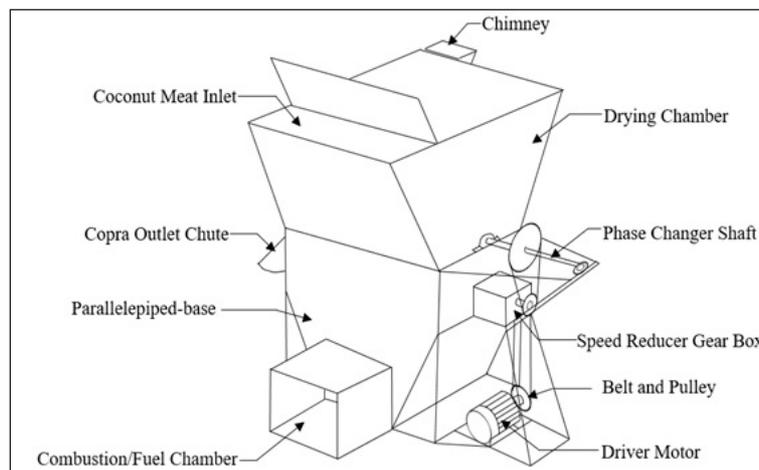
**Figure 1.** Schematic Diagram of the Developed Indirect Heat Copra Dryer with Phase Changer (IHCDPC)
