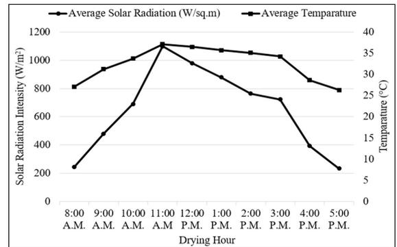
**Figure 7.** Solar Radiation Intensity and Average Ambient Temperature Variation with Respect to Drying Time
