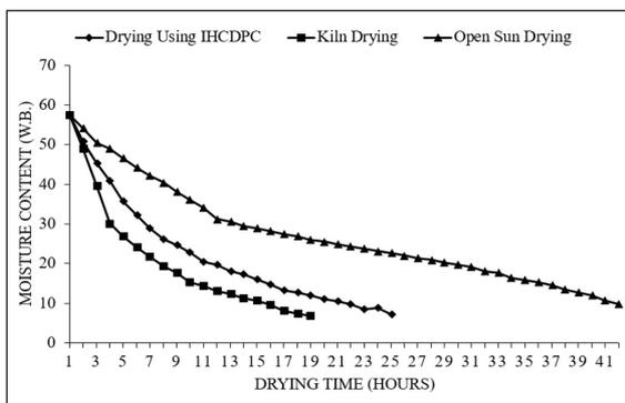
**Figure 6.** Moisture Content Variation with Respect to Drying Time
