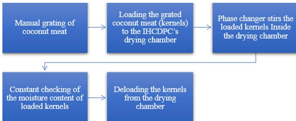
**Figure 5.** Flowchart on How the Coconut was Processed Using IHCDPC
