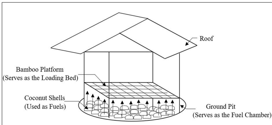
**Figure 3.** Schematic Diagram of a Traditional Kiln Dryer
