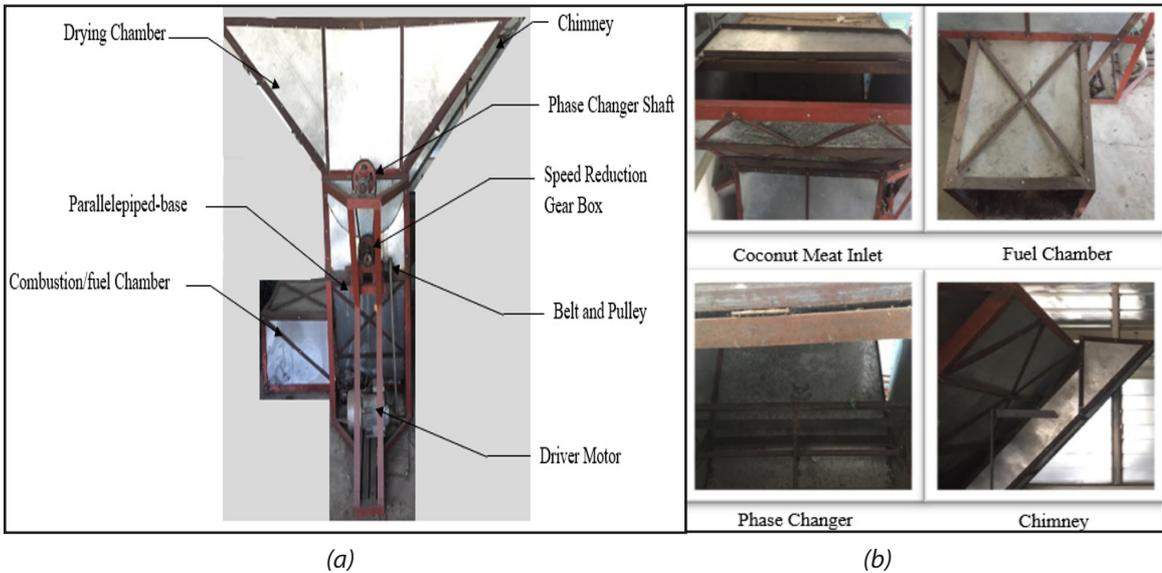
**Figure 2.** Actual Photos of the Developed Indirect Heat Copra Dryer with Phase Changer (IHCDPC)
