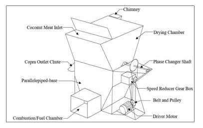
*Figure 1.* Schematic Diagram of the Developed Indirect Heat Copra Dryer with Phase Changer (IHCDPC)
