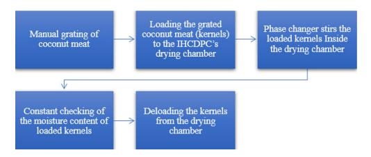
Figure 5. Flowchart on How the Coconut was Processed Using IHCDPC
