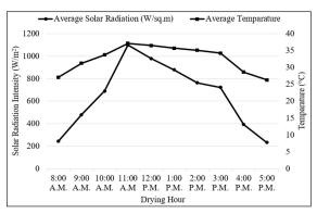
**Figure 7.** Solar Radiation Intensity and Average Ambient Temperature Variation with Respect to Drying Time
