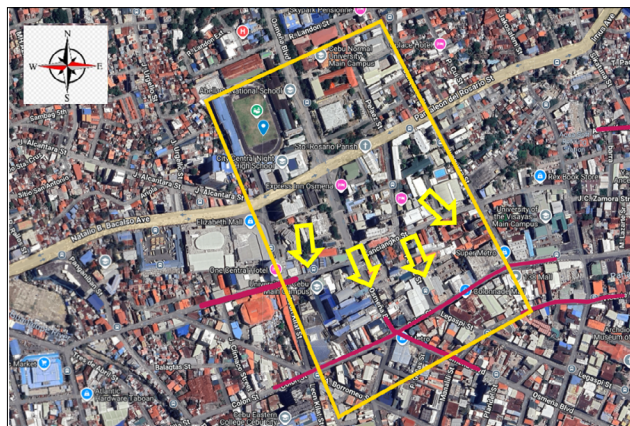
Figure 9. Regularly flooded streets, highlighted in dark red ( Google, n.d. ). Yellow arrows indicate the direction of the street flooding flow.
