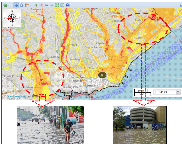
Figure 6. Cebu City's Flood-Prone Areas (DOST-UP DREAM and Phil-LiDAR Program, 2017; Magsumbol, 2021; My Cebu Photo Blog, 2019; einstein143, 2014) are marked as red areas of high susceptibility to flooding.
