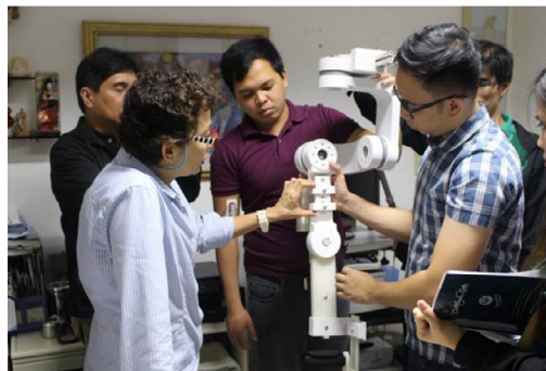
Figure 5. Prototype of the AGAPAY Robotic Exoskeleton ( De La Salle University, 2021 )
