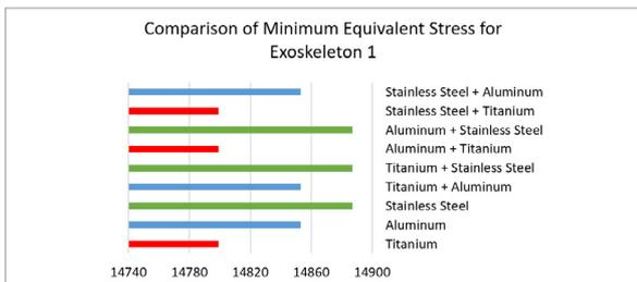
**Figure 12. Comparative Graph of Minimum Equivalent Stress for Exoskeleton 1**
