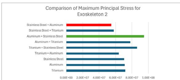
**Figure 20. Comparative Graph of Maximum Principal Stress for Exoskeleton 2**
