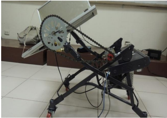
Figure 1. The side view of the dual axis solar tracker with specular reflector (Photo taken by Aliganga, M. inside the Analog Electronics Laboratory of CIT-University).
