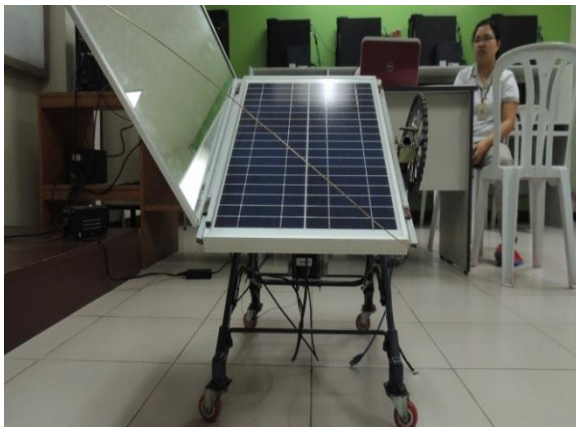
Figure 2. The front view of the dual axis solar tracker with specular reflector (Photo taken by Aliganga, M. inside the Analog Electronics Laboratory of CIT-University).
