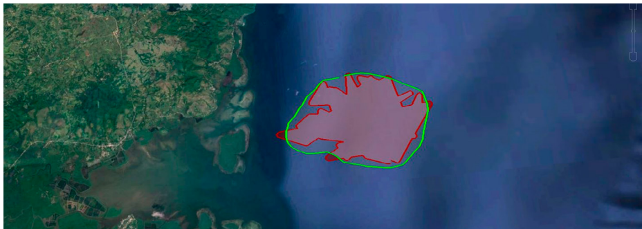
Figure 14. Comparative Visualization of Graham Scan Algorithm Output and Ground Truth Data from Fisherman 10's GPS Tracking
