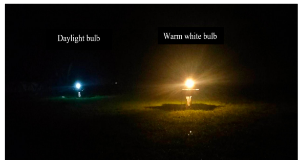
Figure 7. L1T1 (12 watts with Warm White CT) and L1T2 (12 watts with Day White CT)
