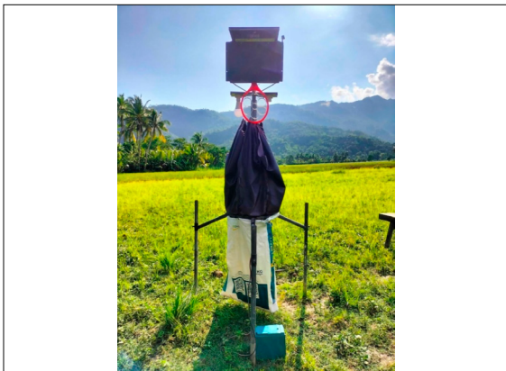
Figure 3. View of the Solar-powered RBB Trap when closed
