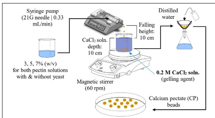
Figure 2. Experimental setup for the entrapment of yeast cells in calcium pectate (CP) beads
