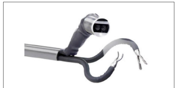
Figure 5. SPORT robotic surgical end effector (Titan Medical Inc., n.d.)
